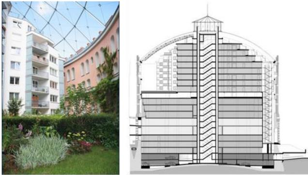
**Figure 15.** A sectional drawing of the new structure designed in the three-armed star form of Gazometre D, and a view from one of the interior courtyards looking towards the outer shell in the upper floors of the living spaces, showing the intersection of the three axes (www.gasometer.org, June 2005).
