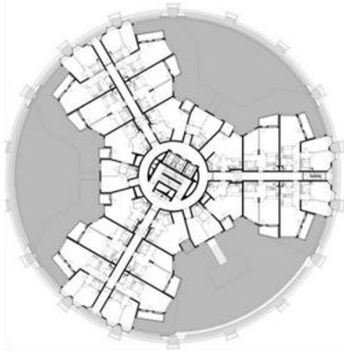
**Figure 14.** Plan drawing showing the inner courtyards created by the new structure designed in the form of a three-armed star for Gazometre D (www.gasometer.org, June 2005).
