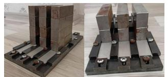
Figure 5. Applying pressure to the adhesive layer using weight
