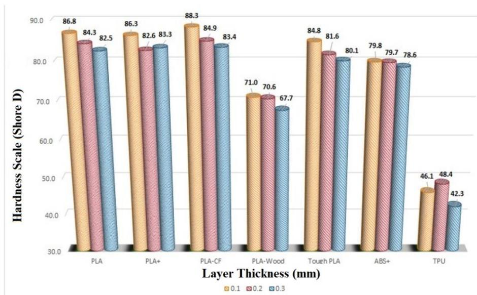
Figure 8. Change of hardness values depending on layer thickness
