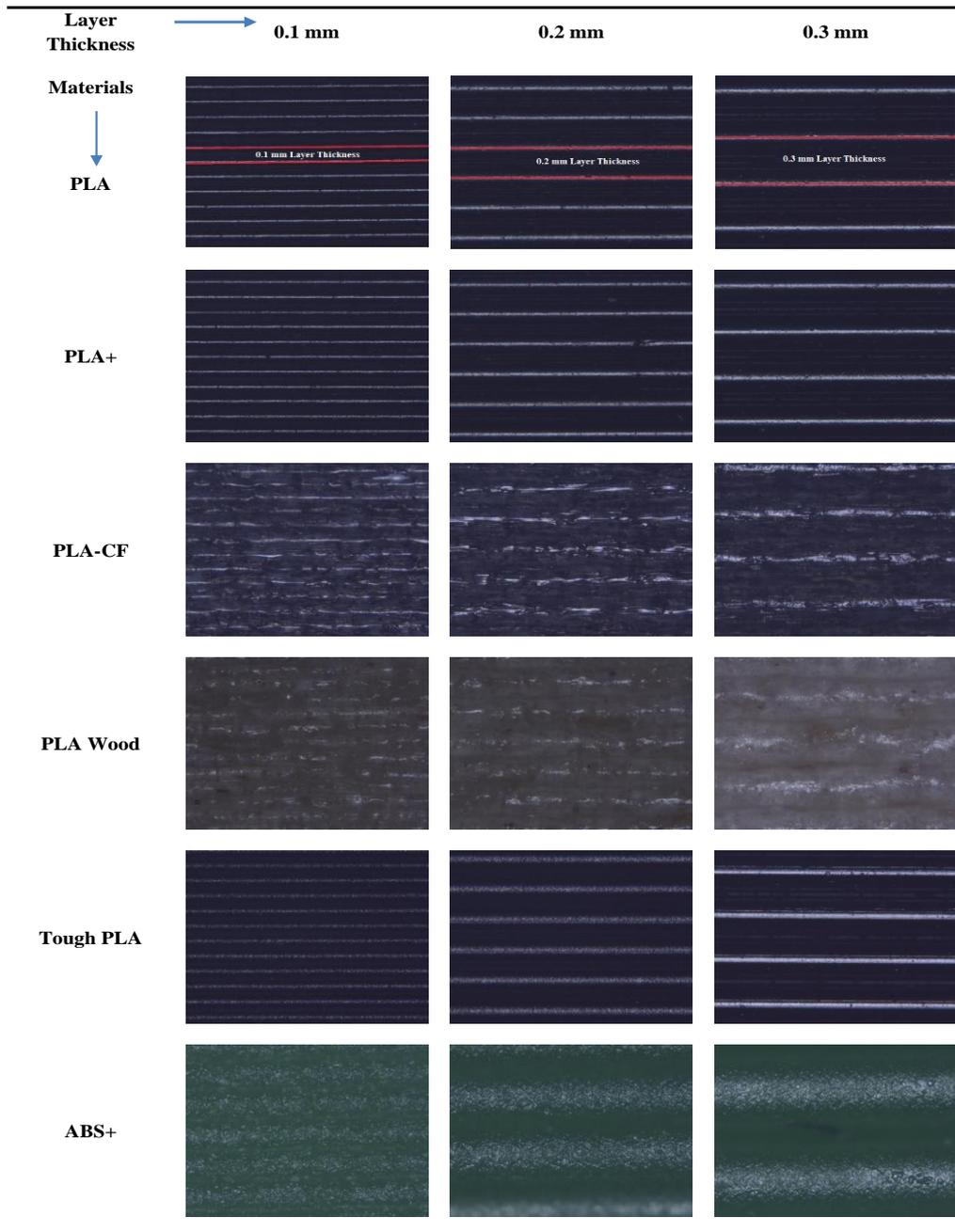
Figure 9. Surface images with an optical microscope (50x)
