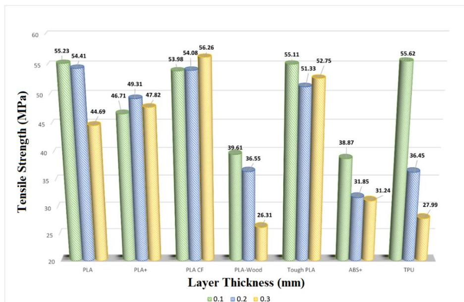
Figure 6. Change of tensile strength with layer thickness
