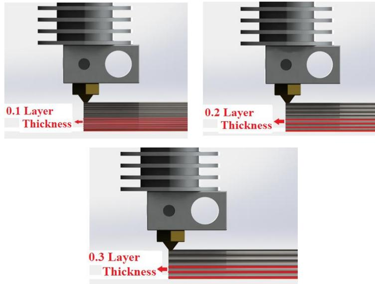
Figure 2. Change of layer thickness applied in 3D printer
