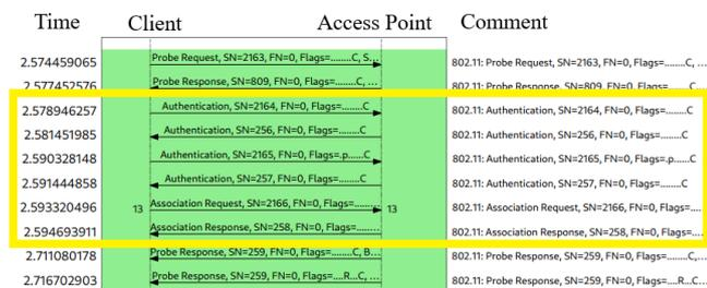
Figure 8. WEP Authentication Connection Process
