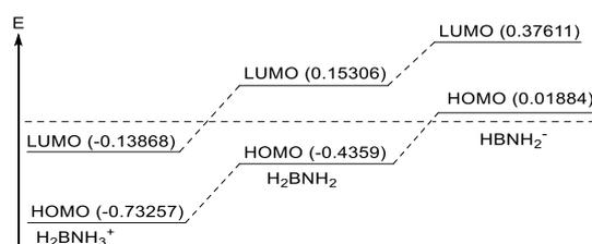
**Fig. 2.** HOMO and LUMO energy diagrams of H<sub>2</sub>BNH<sub>3</sub><sup>+</sup>, H<sub>2</sub>BNH<sub>2</sub> and HBNH<sub>2</sub><sup>-</sup> species calculated at HF/cc-pvdz level.
