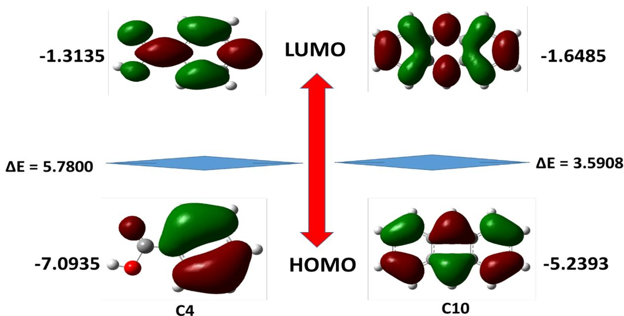
**Figure 3.** HOMO & LUMO energy levels for both Benzoic acid (C4), and Anthracene (C10).
