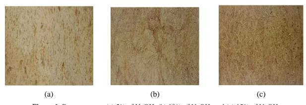
Figure 1. Banana stems; (a) 5% of NaOH, (b) 10% of NaOH, and (c) 15% of NaOH
