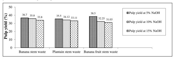
**Figure 2.** Graphical representation of pulp yield of banana, plantain, and banana fruit stem waste pulped with 5%, 10%, and 15% NaOH
