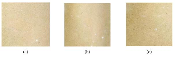
Figure 2. Plantain stems; (a) 5% of NaOH, (b) 10% of NaOH, and (c) 15% of NaOH
