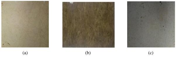
Figure 3. Banana fruit stems; (a) 5% of NaOH, (b) 10% of NaOH, and (c) 15% of NaOH
