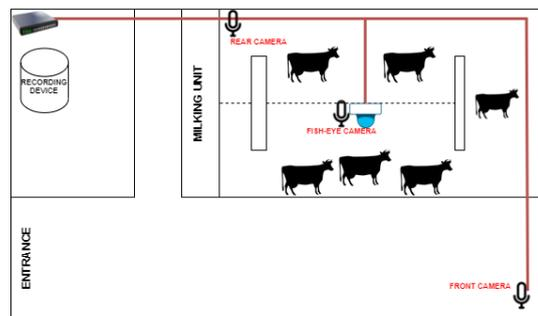
Figure 1. Layout and connection arrangement of cameras and microphones
