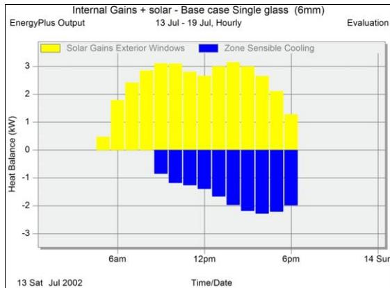
**Figure 6.** Base case room simulation result showing the solar gain through the exterior windows and its effects on cooling load
