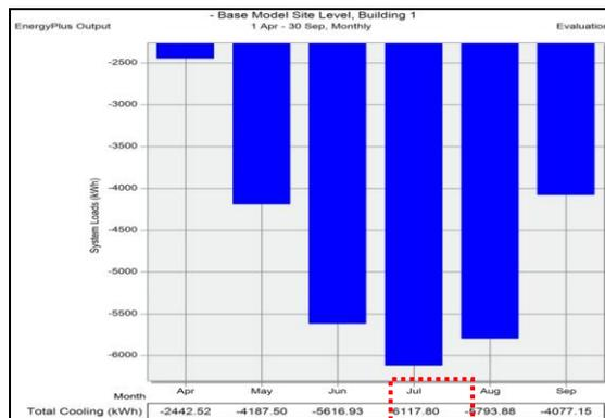
**Figure 17.** Total cooling load result after applying Mahrabiya covering the exterior windows
