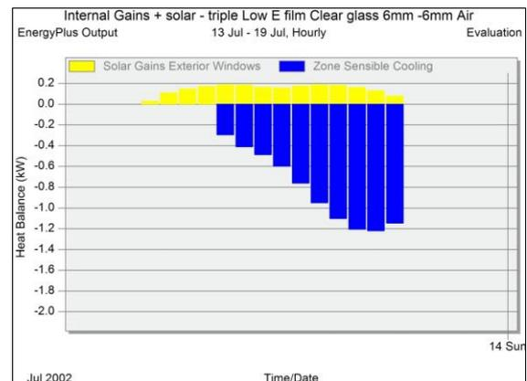
**Figure 9.** Room 3 simulation result showing the solar gain through the exterior windows and its effects on cooling load
