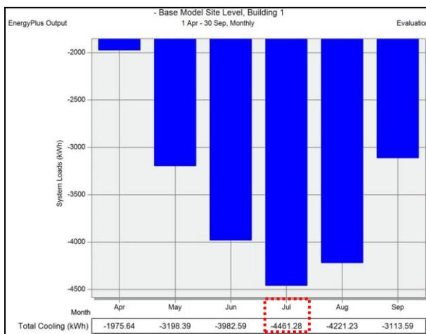
**Figure 20.** Total cooling load result after applying all proposed passive cooling techniques
