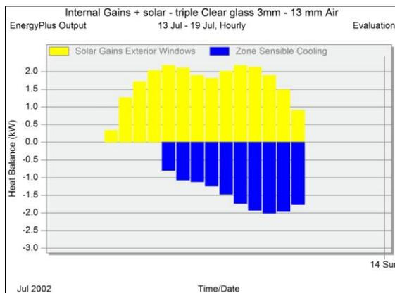
**Figure 8.** Room 2 simulation result showing the solar gain through the exterior windows and its effects on cooling load
