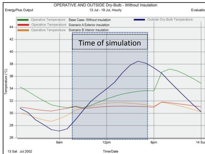
**Figure 11.** Simulation results showing the effect of all roof thermal insulation scenarios on indoor operative temperature
