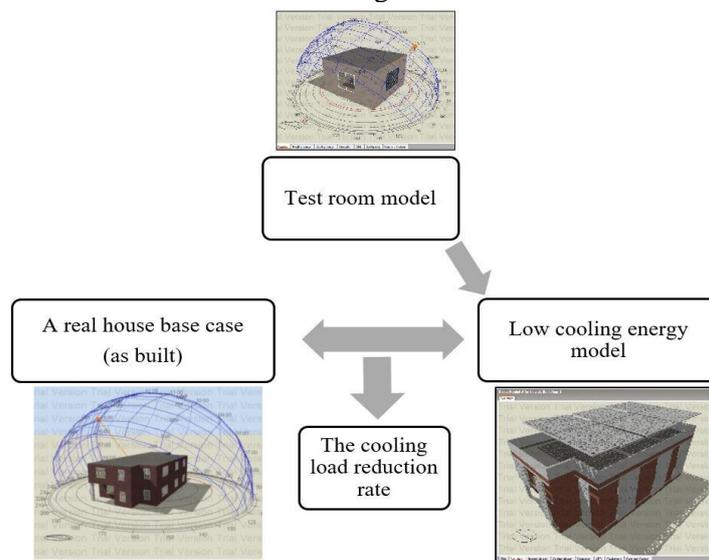
**Figure 3.** A diagram shows the methodology steps of the energy simulation process and the scenarios of each phase
