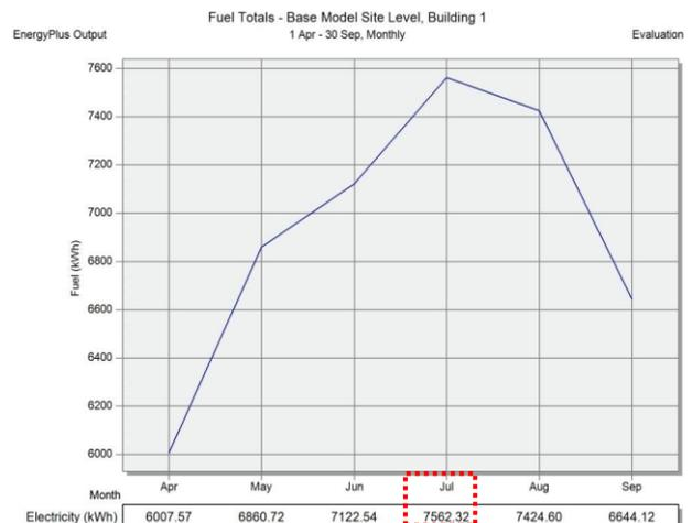
**Figure 21.** Total energy consumption (Electricity) result after applying all proposed passive cooling techniques
