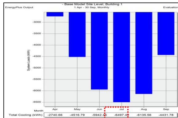
**Figure 18.** Total cooling load result after applying Mahrabiya to cover the flat roof
