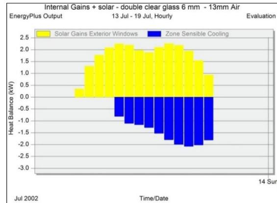
**Figure 7.** Room 1 simulation result showing the solar gain through the exterior windows and its effects on cooling load
