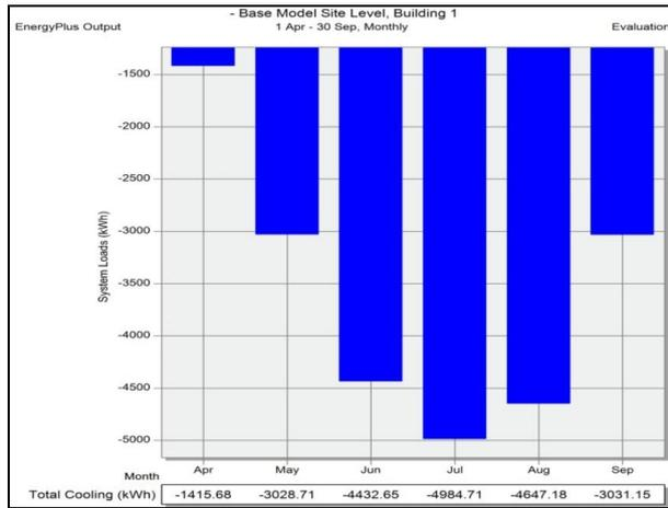
**Figure 19.** Total cooling load result after applying the proposed modify heat gains scenarios
