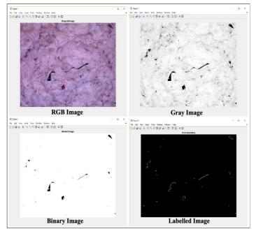
Figure 9. Detection of foreign material in waste cotton bundle
