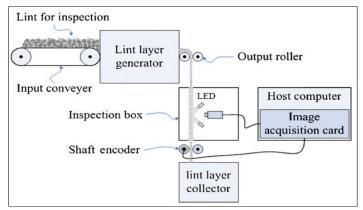
Figure 2. Outline of the machine vision system (Li, Yang, and Wang 2010)
