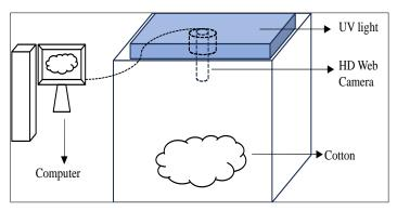
Figure 8. Prototype system design
