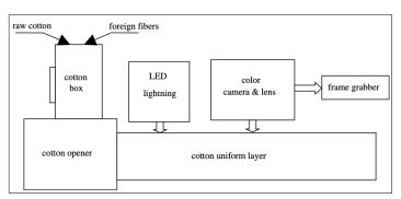
Figure 3. The image acquisition subsystem diagram (Ji et al. 2010)
