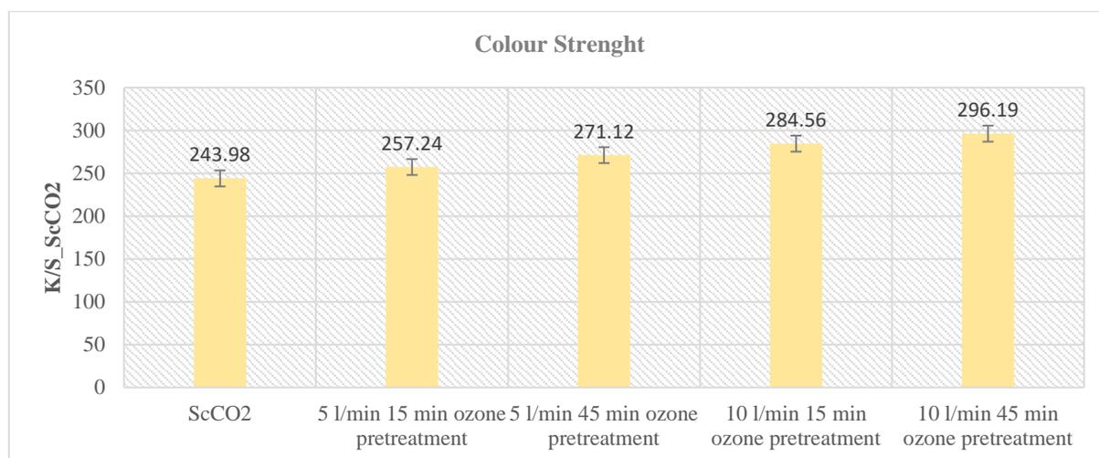
Figure 6. K/S values of pre-treated and untreated fabrics dyed in ScCO<sub>2</sub> medium: K/ScCO<sub>2</sub>:243,98
