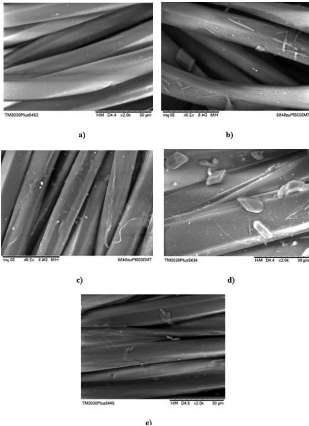
**Figure 7.** SEM images of raw and dyed fabrics; a) Sem image of raw fabric, b) SEM image of conventional dyed fabric, c) SEM image of fabric dyed in  $scCO_2$  medium, d) fabric dyed in  $scCO_2$  medium, pre-treated with ozone for 45 minutes at a flow rate of 5 L/min ozone gas, e) fabric dyed in  $scCO_2$  medium, pre-treated with ozone for 45 minutes at a flow rate of 10 L/min ozone gas
