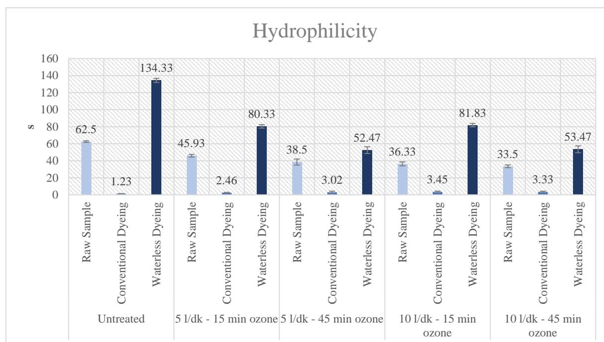
Figure 4. Hydrophilicity test results of the samples
