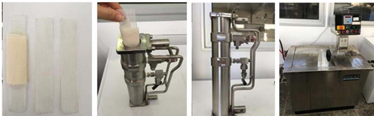
Figure 3. ScCO<sub>2</sub> dyeing machine and tubes [16]
