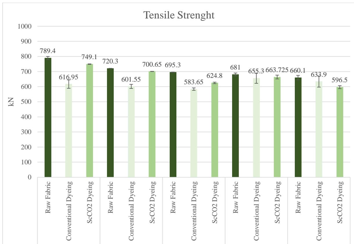
Figure 8. Tensile strength values of the fabrics
