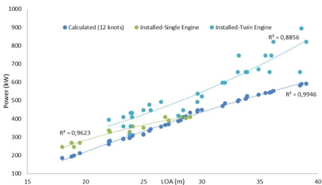
**Figure 3.** Calculated power-installed power comparison for Bodrum Gulets
