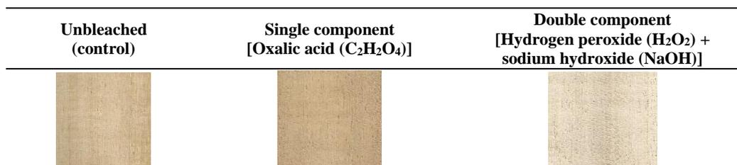
The measurement results for all tests are presented in Table 6. According to these results, changes were observed in  $L^*$  values with both chemicals. The lowest increase in  $L^*$  value was 2.20% in the single-component while the highest increase was 13.16% in the double-component. The highest  $L^*$  value was observed in the double-component (78.18) while the lowest was found in the control samples (69.62).
