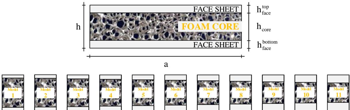
Fig. 4. Cross-sectional scheme of the 11 sandwich plate models.
