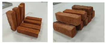
Figure 2. Waste marble powder doped brick sample
