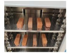
Figure 3. Drying the samples in an furnace
