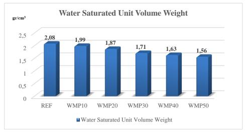
Figure 6. Graph of water saturated unit volume weight
