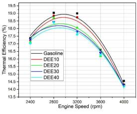
Fig. 5. Changes of thermal efficiency
