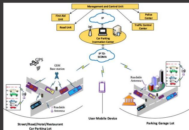
Figure 3. Cloud-based smart parking system and IoT supported smart city architecture
