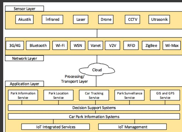
Figure 2. Smart parking system layer and components
