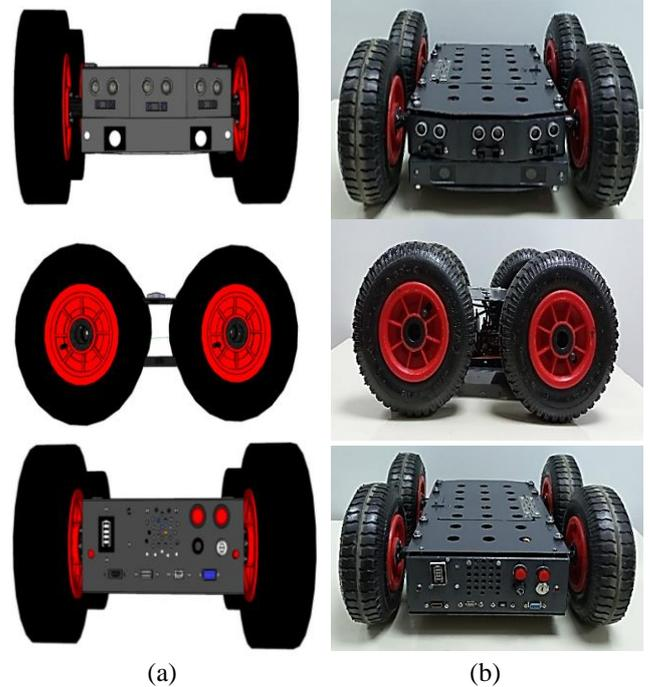
Figure 3. Mobile robot (a) 3D drawing view and (b) Realized view
