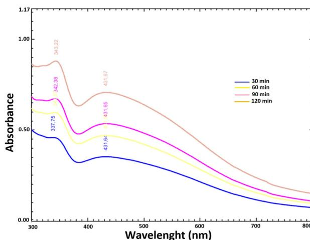
Figure 1. Time-based UV-vis absorption spectra of AD-AgNPs
