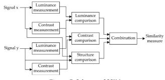
Figure 5. Schema of SSIM
