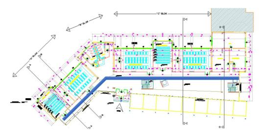
Figure 9. A Schematic Representation of Fresh Air Delivery Through the Atrium.
