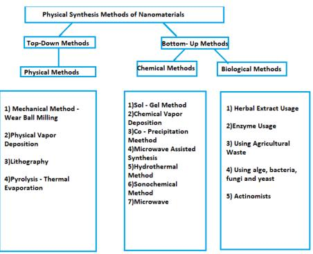
Figure 1. Synthesis methods of nanoparticles [13–19].
