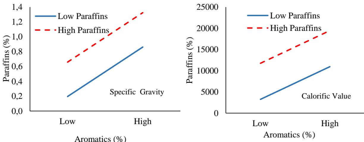
Figure 4-b. Effect on fuel specific gravity and calorific value
