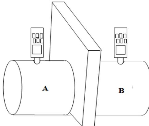
**Figure 3.** Experimental setup for sound absorption coefficient (SAC) test
