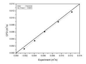
Figure 19. Comparison of rectangular labyrinth weir discharge
