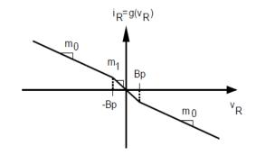
Figure 3. Three-segment piecewise-linear (PWL) *v-i* characteristic of the Chua's Circuit (Kennedy 1992).
