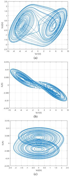
Figure 13. Phase portraits of the circuit: a)  $V_{c2}$  vs.  $V_{c1}$ , b)  $i_L$  vs.  $V_{c1}$ , and c)  $i_L$  vs.  $V_{c2}$ .
