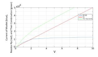
Figure 8. a) Resistor  $R_p$  characteristic shown in red, b) The BF245B JFET characteristic for V<sub>GS</sub>=0 Volt shown in blue, and c) Their combined characteristic shown in green.
