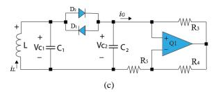
Figure 2. Three examples of the Chua's diodes taken from a) (Matsumoto 1984), b) (Kennedy 1992), and c) (Xu 2015).
