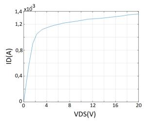
**Figure 6.** *V*<sub>DS</sub>-*I*<sub>D</sub> characteristic of BF245B JFET obtained experimentally.
