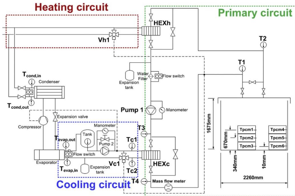
Figure 3. Schema of thermal storage system [12]
