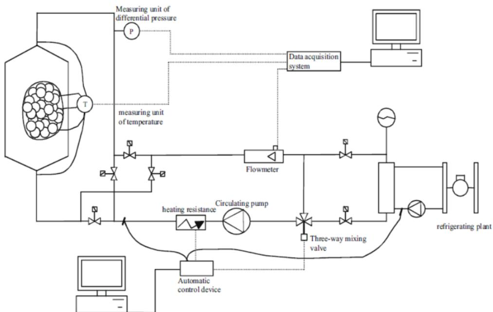
**Figure 4.** Encapsulated thermal energy storage system [14]
