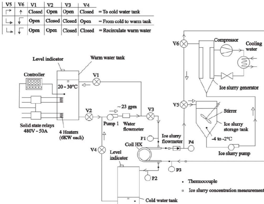
**Figure 6.** Laboratory scale ice slurry thermal energy storage system [18]
