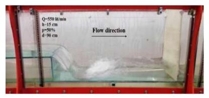
Figure 3 - Vertical drop equipped with a screen and hydraulic jump formation
