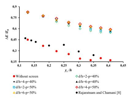
Figure 7 - Effect of screens on relative energy dissipation
