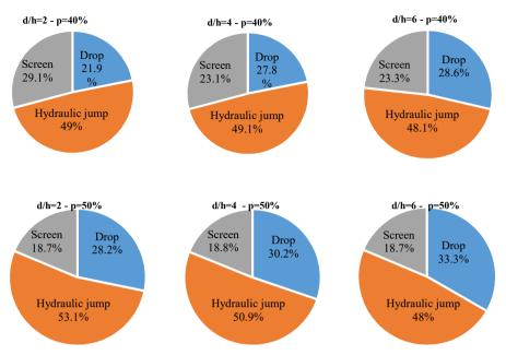
Figure 11 - Variation of energy dissipation percentage for different components
