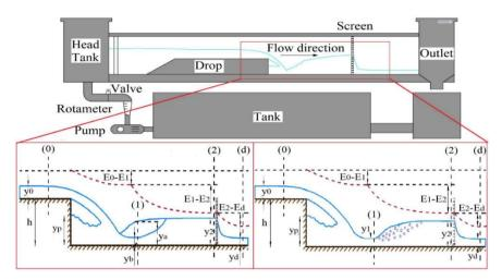
Figure 1 - Schematic of experimental setup and water circulation system
