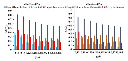
Figure 10- Contribution of different components in energy dissipation
